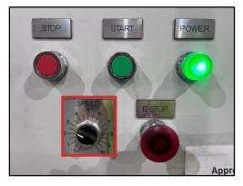
4. It is recommended that the machine operate at speeds between two and three to ensure safety and stable product sorting. However, the grading process department can use the speed of ten due to the fast pace required for grading cloth products.
