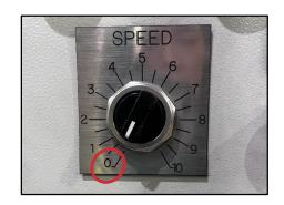
3. Press the **"STOP"** button or turn the knob horizontally and counterclockwise on the conveyor control panel.
