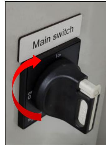
3. Turn on the main power switch near the Boxer's top.
