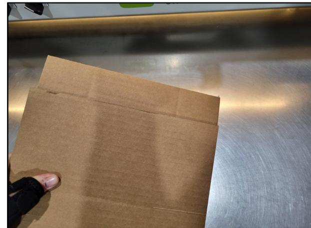
5. Place the box on the table with the flap leading into the machine. Slide the box forward until it cannot go further, triggering the gluer to activate. Hold the box steady while the glue sets, which will take about 15 seconds.
