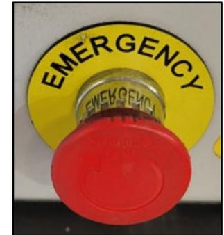
**Note:** If an emergency occurs while using the boxer and the Emergency Stop is used, press the flashing exclamation button to reset it.
